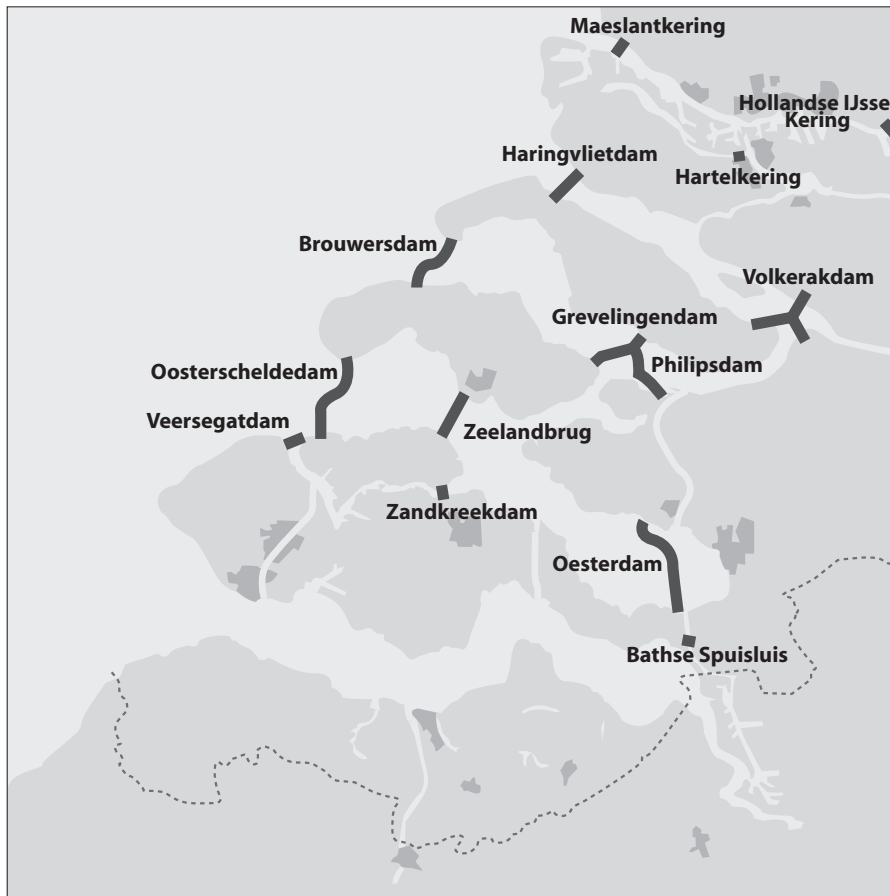
Figure 1.5 The final design of the Delta Plan, with three movable storm surge barriers, one bridge, and nine dams
